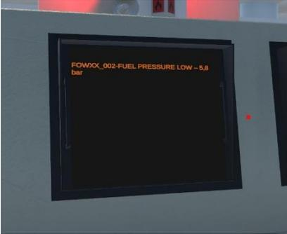
A close-up of the top monitor showing the alarm message: "FOWXX_002-FUEL PRESSURE LOW - 5.8 bar".                                                                         |
